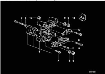
In particular - the part we're interested in is the piece exploded off to the lower right, with screws 2 & 3 going into it. This is where you adjust the rocker arm endplay. (Images from MAX-BMW's website – great on-line parts catalog)
