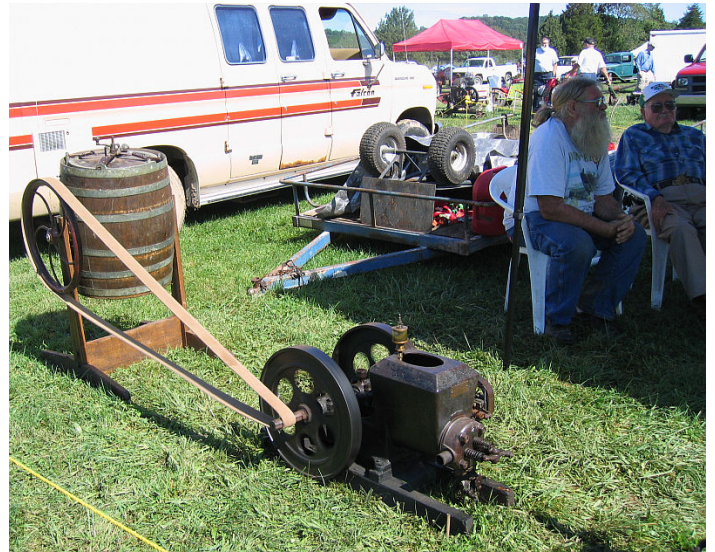
Hit and Miss engine powered washing machine – yeah, it's running..
