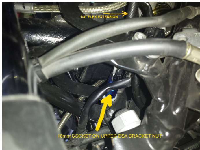
Flex extension used to get to front mount Torx. (photo M. Agnello)
