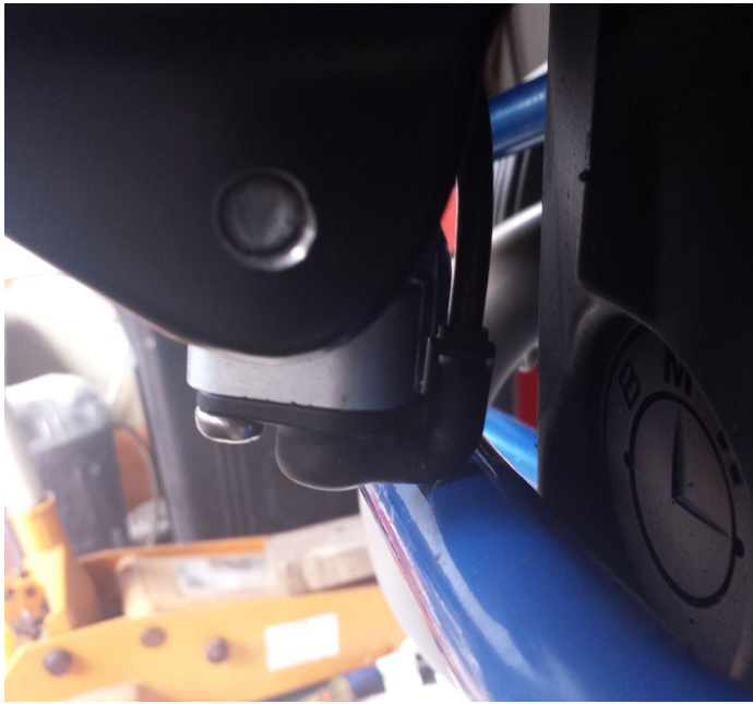
The wrong way to mount the ESA connector. (photo M. Agnello)
