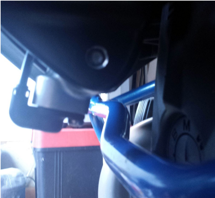
The right way to mount the ESA connector. (photo M. Agnello)
