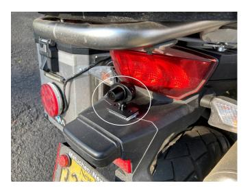
Rear camera does not interfere with visibility of Tail light. Both cameras are IP68 water-proof. Camera cables are about 1 foot but have approx 4 foot extensions. Camera connectors and wire extensions to DVR appear to be secure and waterproof.
