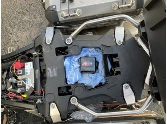
Both DVR and 12VDC power block are located under rear seat area (where my tools use to be located. Scrap blue towel is used for cushioning. Power module has + and – battery connection and yellow wire for ACC switched power. You must locate a ACC lead which tells DVR to power up when your bike starts.
