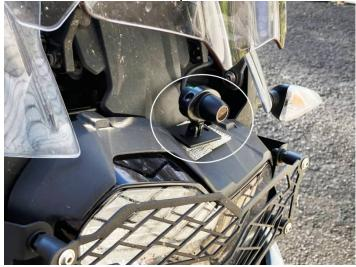
Front camera is wired to the DVR located under seat. Looks like a deer Whistle. I used of 3M Duel Lock instead of 2-sided foam tape; this allows camera to be adjusted right to left later. Camera has hinge for up-down adjustment.
