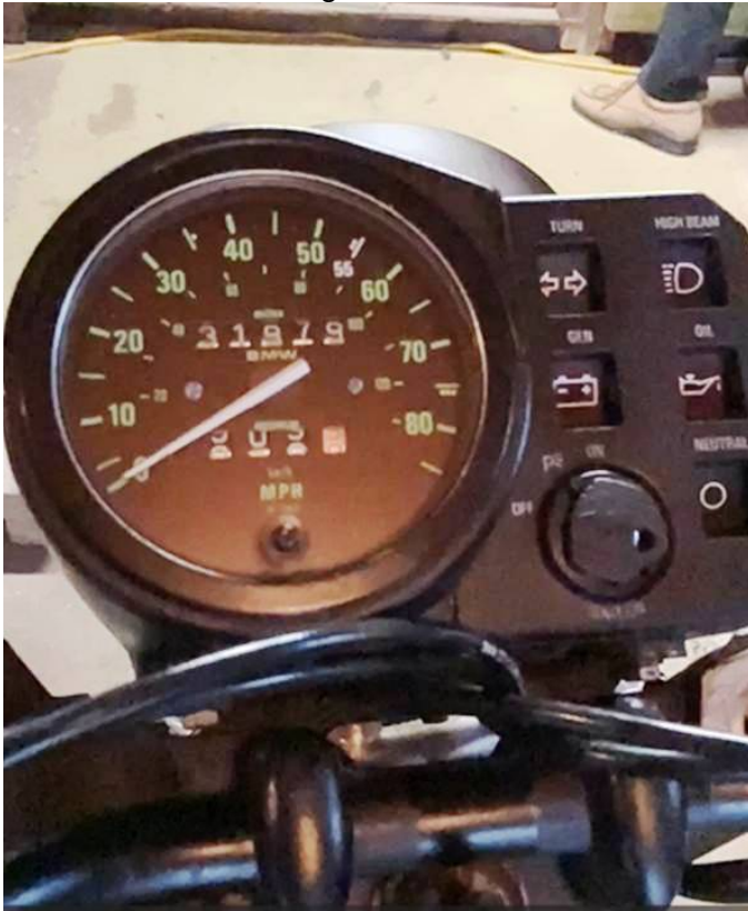
Original Speedometer showing 31,979 miles. Notice how the speedometer fits into the headlight/instrument cowling.
