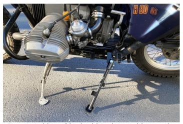
Down position of both old and new side stands. The OEM stand is located way under the engine cylinder making it hard to set.
